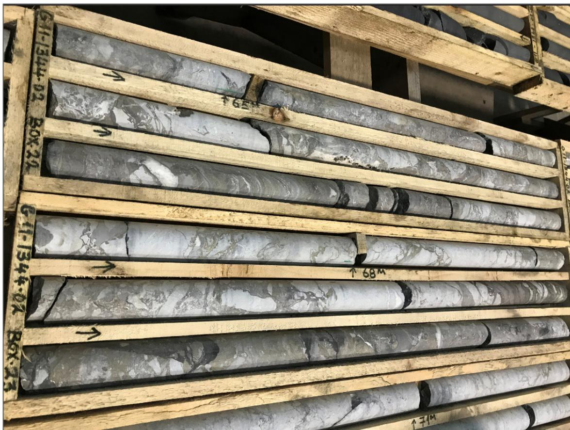
**Figure 12.1** Drillhole G11-1344-02: Core trays showing interval ~64.8 to ~70.5 m, with mineralogical assemblage consisting of pyrite, sphalerite and minor galena
