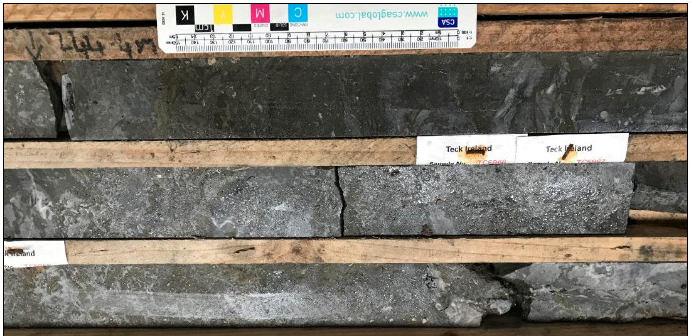
Figure 12.2 Drill hole TC-2638-099: high-grade interval 244.80 – 246.24 m (length weighted average Zn = 15.72% and Pb = 6.42%) (Source: CSA Global, 2018)
