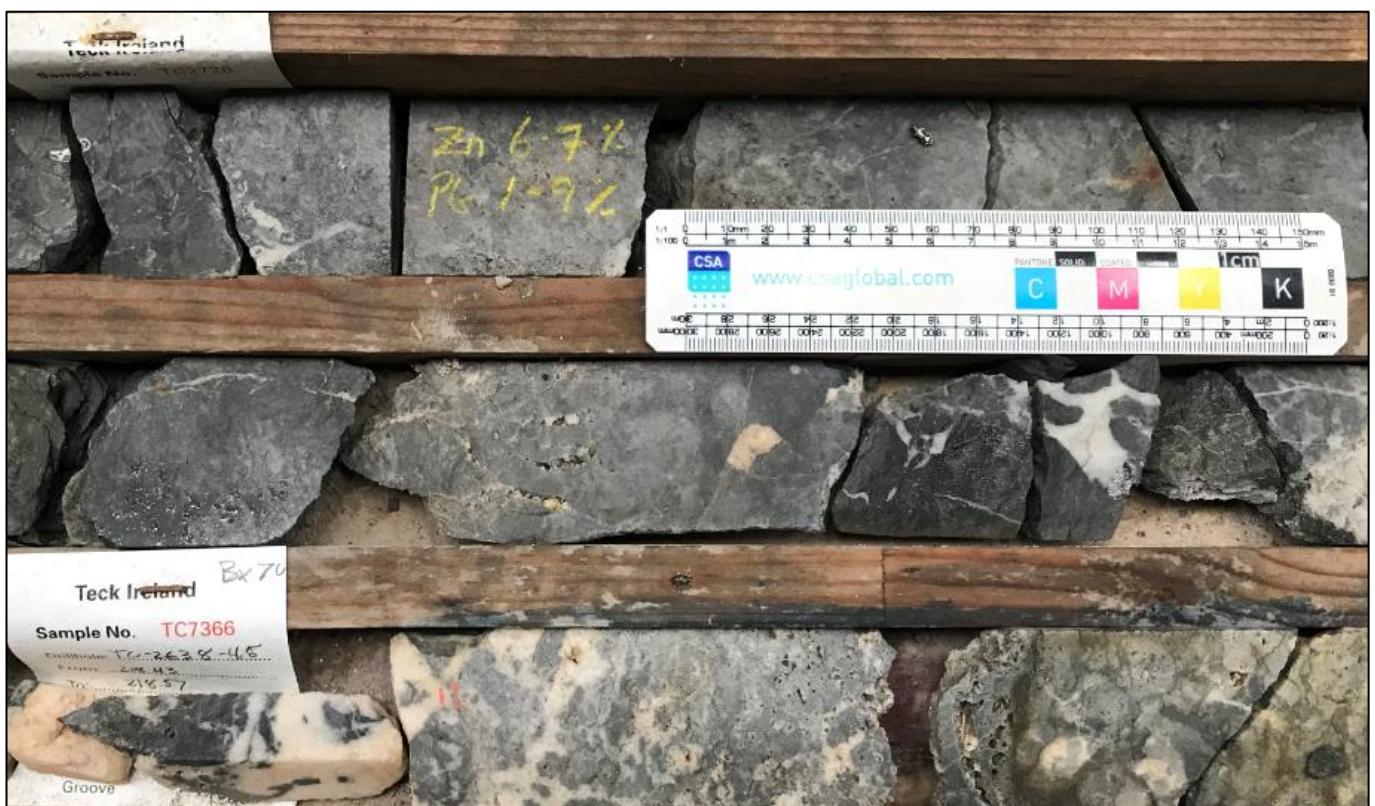
Figure 12.1 Drill hole TC-2638-045: high-grade interval 216.10 – 216.55 m (Zn = 6.76% and Pb = 1.98%) (Source: CSA Global, 2018)
